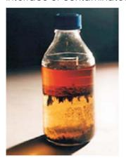
Fungal hyphae and other debris from the surface of a diesel fuel filter which blocked in service.
